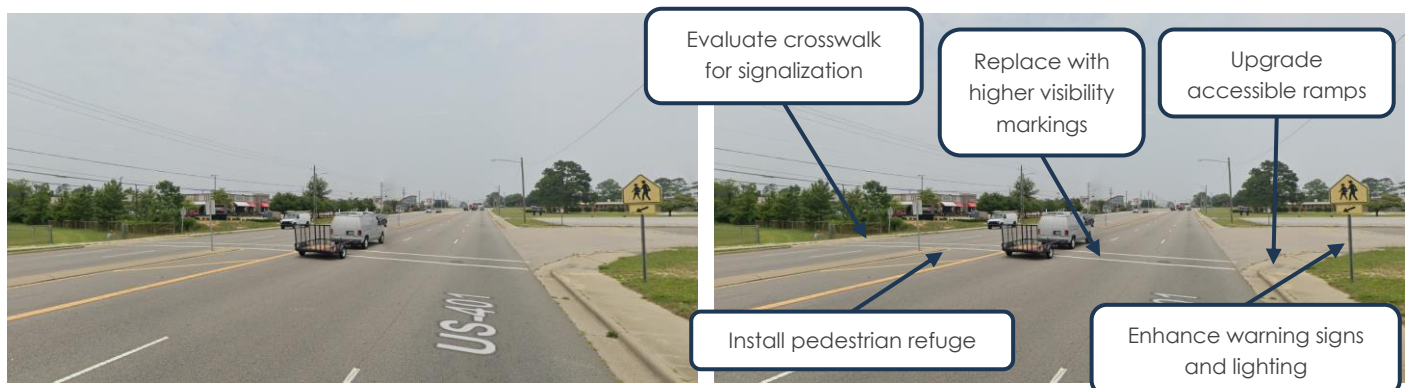
Figure 5: Example for improving uncontrolled pedestrian crossings on higher-speed arterials (image source: Google Maps)
