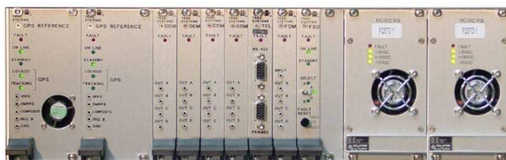
Figure 1-23: TRAK 9100 Simulcast Site Reference – Provides the simulcast system 1 PPS, 5 MPPS, and 1 PPS + 5 MPPS composite signals to synchronize the simulcast transmissions.
