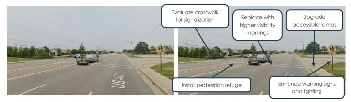
Figure 5: Example for improving uncontrolled pedestrian crossings on higher-speed arterials (image source: Google Maps)
