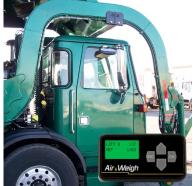
container. After each lift, the driver can simply drive to the next bin and complete the lift without pushing buttons on the scale. To document the lift with a weight receipt, the driver needs only to press a single button on the display.
