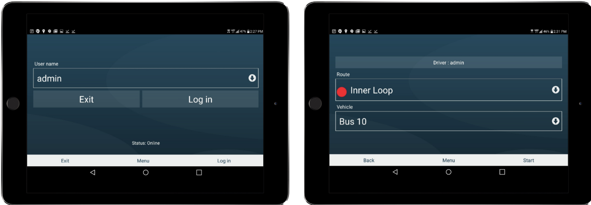
The driver app interface allows operators to choose a route and vehicle to begin the day
